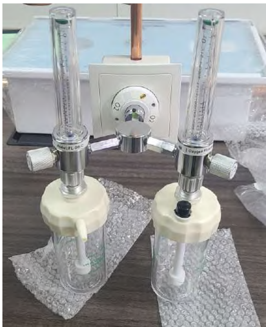
DOUBLE FLOWMETERS SAMPLES CONNECTED TO A TERMINAL UNIT
